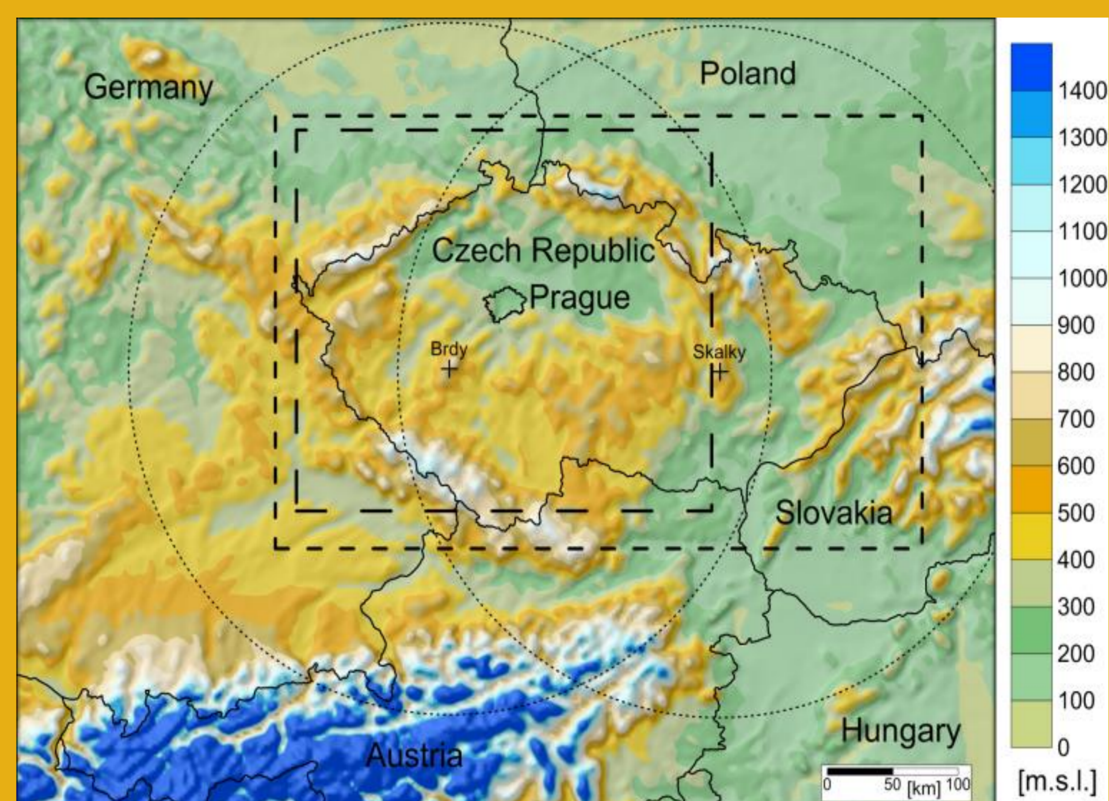
Fig. 1. The model domains with the resolution of 2.8 km (larger) and 1.1 km with topography above sea level in m (see legend). The positions of the Brdy and Skalky radars (black triangles) and the areas covered by the radar data assimilated into the model (dashed circles) are marked.
