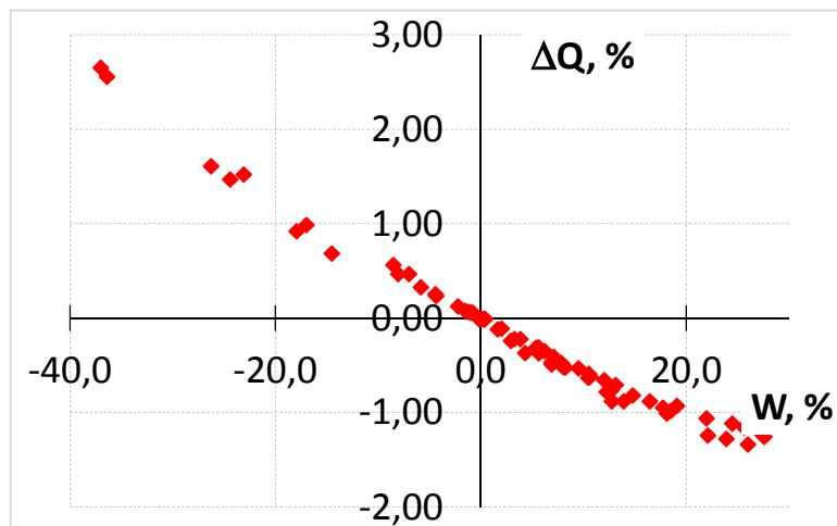
Uncertainty in solar irradiance due to water vapor profile is less than 0.2%
