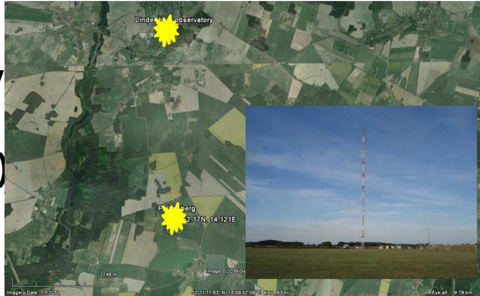
At **Falkenberg** site (6 km to the south from **Lindenberg**) BSRN-like radiative measurements are available: all components of shortwave radiation (direct, diffuse, global, reflected shortwave irradiance)
