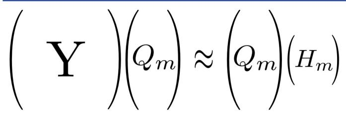
Figure 2: Schematic representation of the relationship and dimensional size between the Arnoldi matrices and the full matrix Y. The Krylov subspace can be much smaller than the original system.
