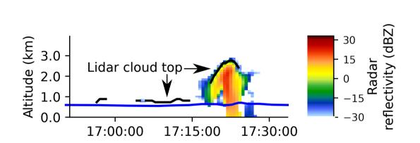
Fig. 4: Example scene from ICON LEM. Forward simulated radar signal and lidar cloud top height from meteogram output.
