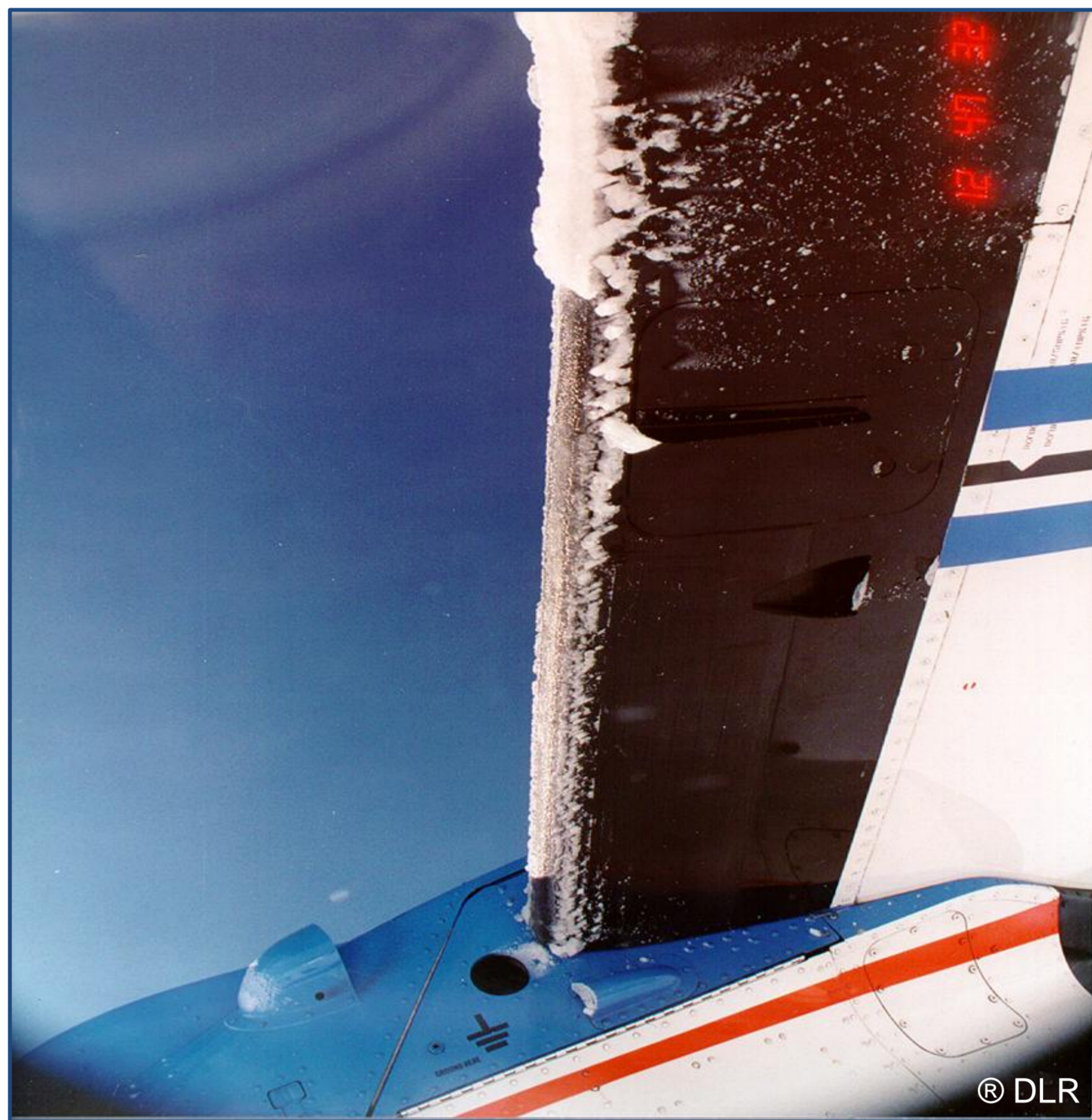
Fig. 1: DLR Dornier-228 research aircraft after the encounter of icing conditions.
